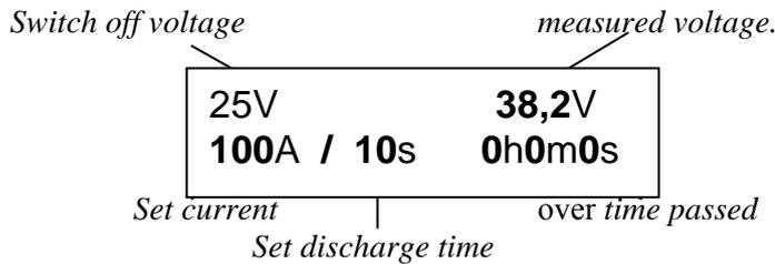
Press START for a measure that equals in all the parameters of the former measure.
